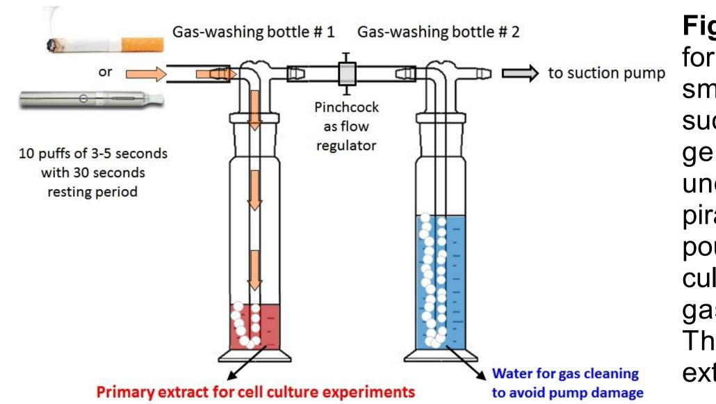
**Fig. 1:** Experimental setup for simulation of cigarette smoking or vaping. The suction pump on the right generates an adjustable underpressure which aspirates the smoke or vapour and bubbles it into the culture medium in the left gas-washing bottle # 1. This yields the primary extract.
